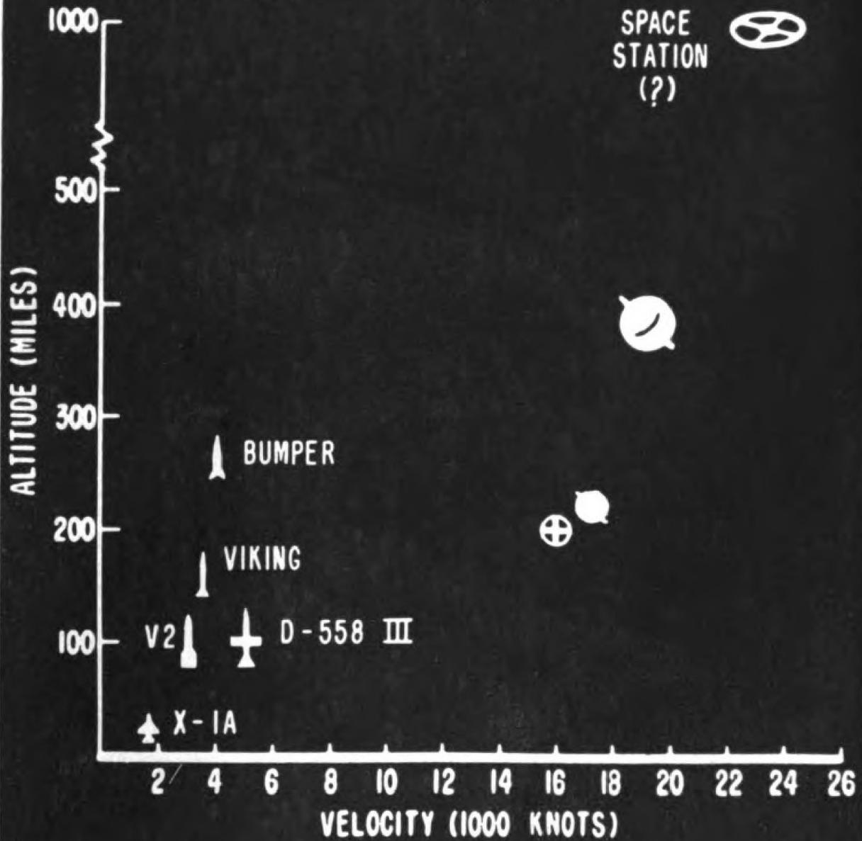
Above chart shows progress being made with rockets and illustrates tremendous speed which must be attained to establish a space station which would orbit the earth. A three-stage Redstone rocket was fired over Atlantic in late 1956. It traveled 3000 miles, went 400 miles up.
